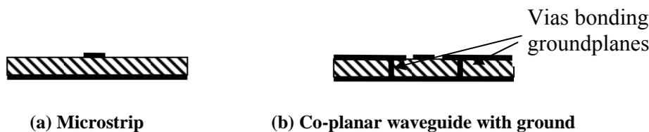
**Fig 10: Transmission line configurations**
