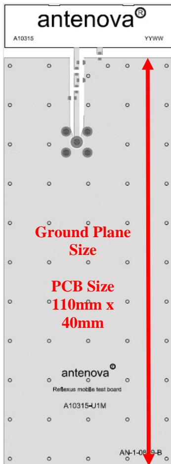
Performance variation vs Gnd Plane Length (GSM850, GSM900)
