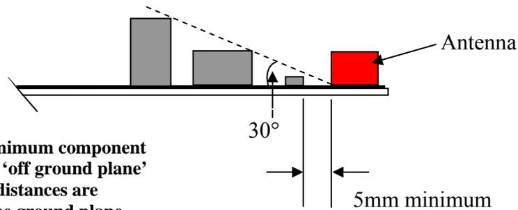
**Fig 1: Typical minimum component clearances to the 'off ground plane' antenna, but the distances are measured from the ground plane edge.**
